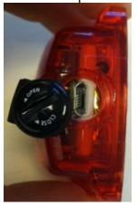
It is important to keep the cap fully locked at all times because this cap blocks water from wetting the inside of the monitor. However, this cap, even when locked, is VERY easy to pop open during data collection (e.g. inadvertently twist it open when changing clothes). Therefore, in addition to locking the cap before mailing the monitor, study staff needs to remind the subjects and parents to keep an eye on the cap and make sure it stays in.
