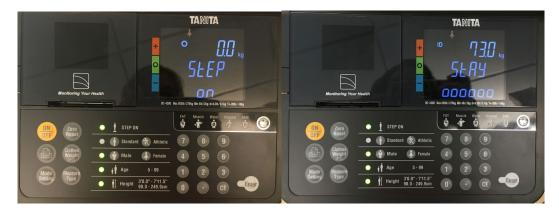
8. The subject will then be measured for the body composition data. The process is complete once there is a beep and the weight in kilograms, kilograms of body fat, and body fat % is displayed on the control box.
