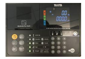
7. "88888 kg" will blink until the machine is ready for use. Then the control box displays "Step On", prompting for the subject to get on the electrode pads. The feet should make contact on all 4 electrode surfaces.
